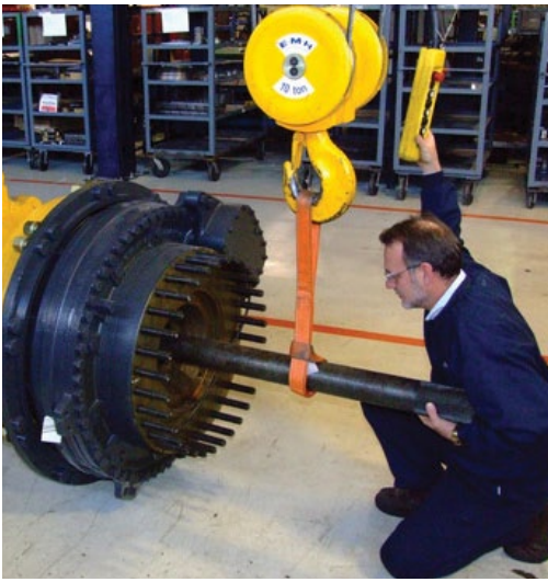
Inspecting a pivot shaft at SRC
